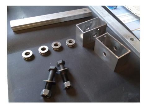
The main point with this gimbal is that the thickness of two bearings and whatever you use as a stick add up to the internal width of the aluminium – in my case 9 + 9 + 10 + 6 = 34mm, which is the inside width of 80 x 40 x 3mm extrusion.
