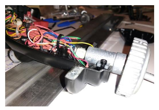
The grip's flange was cut at an angle, and a pipe clamp holds the flat surface against the aluminium stick. It may not look like it, but it's rock solid.
