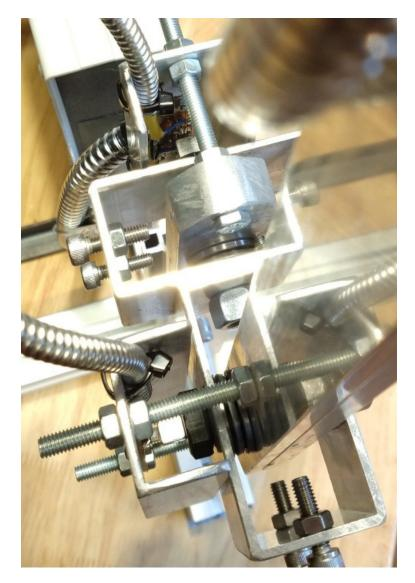
The distance between the sensor and the magnet sets sensitivity. These sensors and magnets needed to be very close for my chosen range of movement, but there might be better sensors and stronger magnets available.
