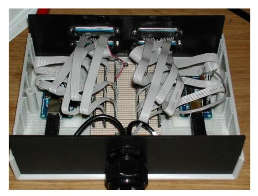
Each BU0836 has two 25 pin sockets, each with the pinout below – which allow devices to be disconnected easily, whilst still sharing input pins.
