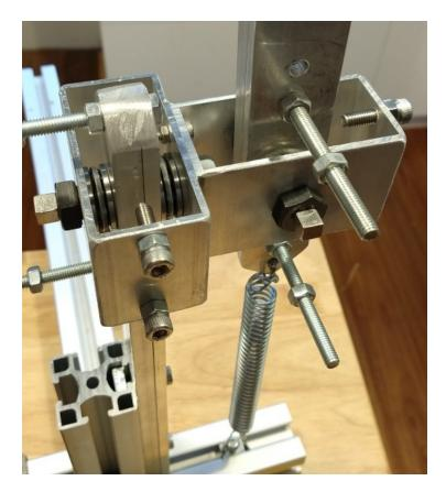
You can also see the 5mm neodymium magnets, limit screws, and centring spring above. The long bolts are for mounting the sensors and sensor covers.
